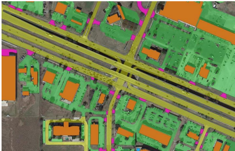
Figure 5.6. Ecopia classification distinguishes the public road system from driveways, parking lots and buildings
