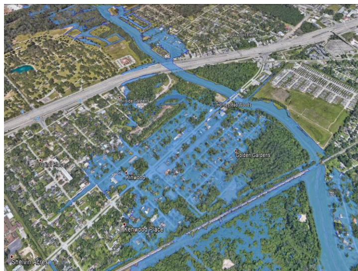
Figure 3.5 Flood Inundation Map showing inundated roads at bridge locations Source of Figure – National Weather Service
