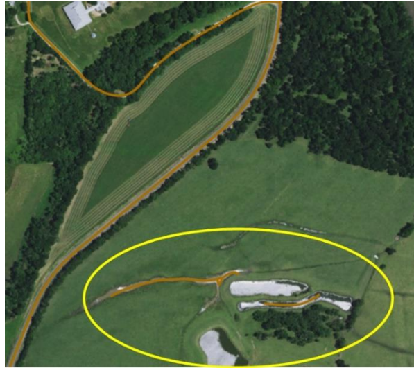
Figure 5.8. Spurious road features in a field identified by the ESRI Road Extraction Deep Learning model.
