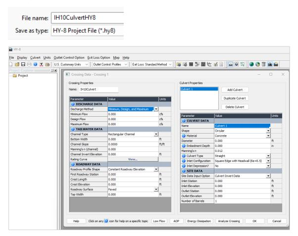
Fill in the input data for the culvert as shown below. Note that this is one culvert with two barrels.
