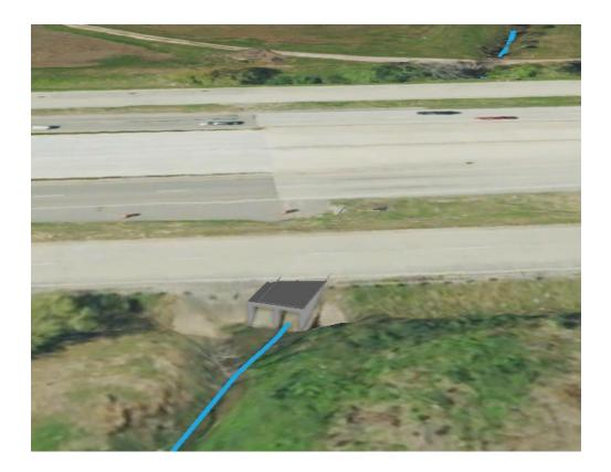
If the road surface polygon is digitized and LIDAR elevation points lying within that polygon are obtained, the result appears as:
