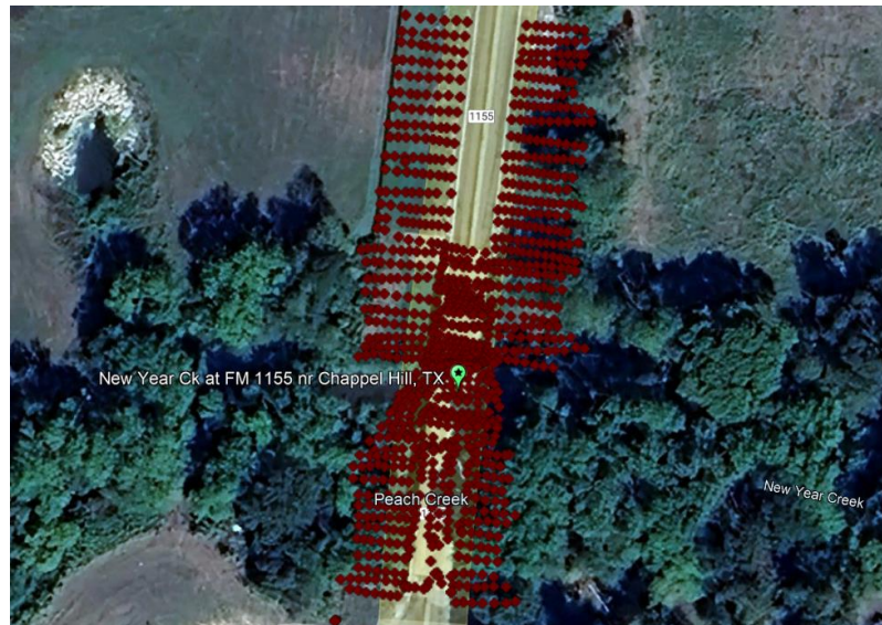
Figure 5. Manually surveyed point cloud around the New Year Ck at FM 1155 nr Chappell Hill, TX bridge location to create higher quality bathymetric elevation models near the bridge where Lidar struggles to acquire data.
