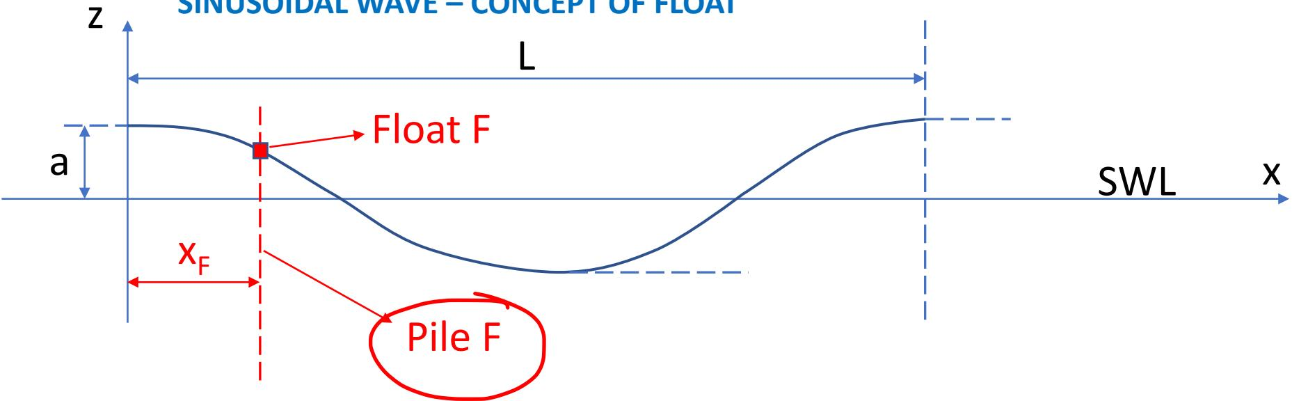
Float F can follow the wave surface at  $x = x_F$  without friction
