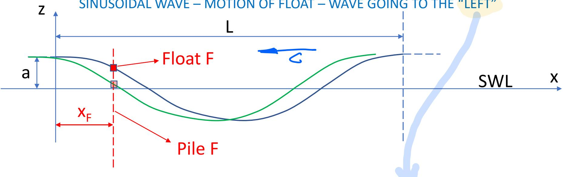
$$\underline{\eta_F(t)} = \underline{\eta(x_F, t)} = \underline{a \cos(kx_F + \omega t)}$$
